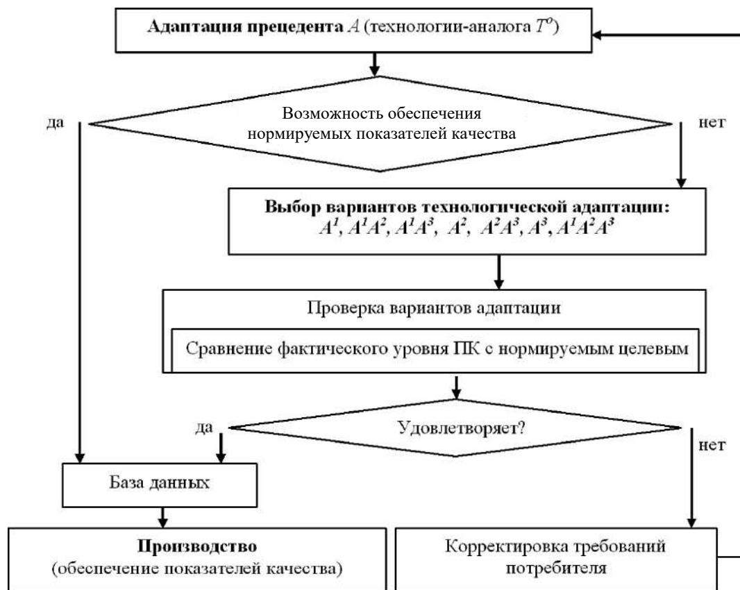
Fig. 1. An algorithm for technological adaptation of the metal products quality indicators based on a precedent in the technological system
